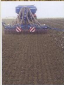
The combination of Knight 'M' Press and Rabe Megaseed produces a versatile single pass till and drill solution.
