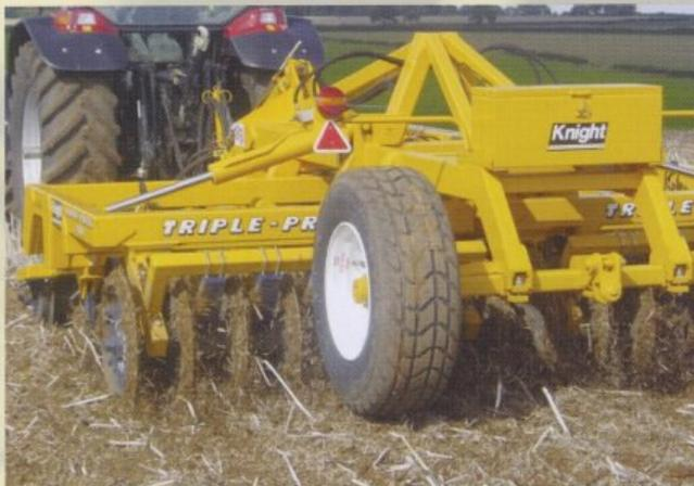
A heavy duty press cultivator designed for primary or secondary cultivation with two rows of tines or discs followed by the Dutch Tine levelling system and a double row of 700mm diameter 'Revolver' press rings.
