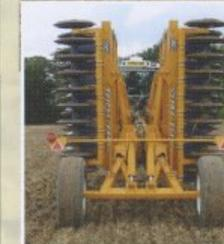
A heavy duty primary cultivator combining discs and tines to give good trash control and soil loosening without forming a pan.
