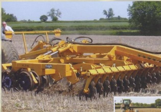
Combines discs, tines and press rings to provide a single machine, equally at home as a primary cultivator in a minimum tillage solution or a secondary cultivator in a plough based system.
